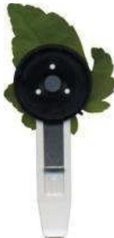
Figure 18: Correct placement of the clip on the leaf / Placement correct du cache sur la feuille, source: Hansatech Instruments Ltd, 2006
